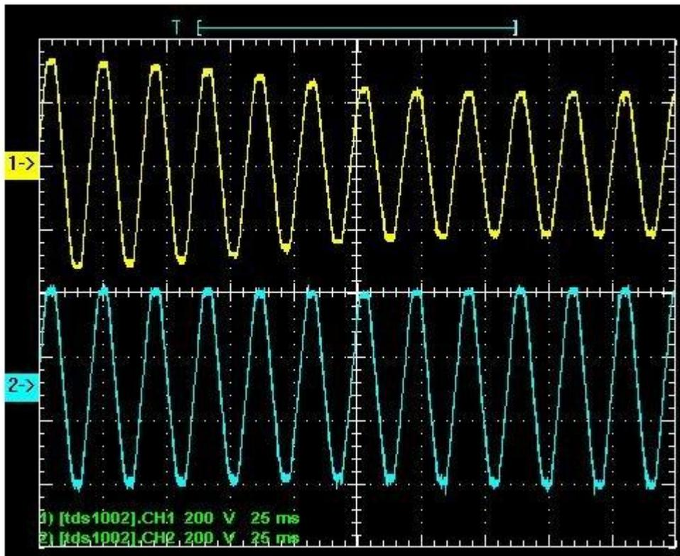
As we can see in the above waveform, input voltage (channel 1 – yellow) is dragged down from high voltage to low voltage within 0.2sec, but the output voltage (channel 2 – blue) remains steady.
