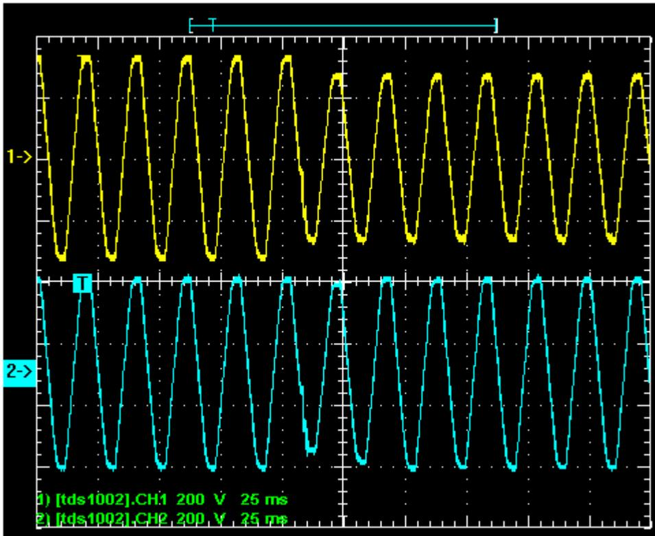
The input voltage (channel 1 – yellow) stepped down from high voltage to low voltage in no time, and the output voltage (channel 2 - blue) corrected immediately in the next cycle.
