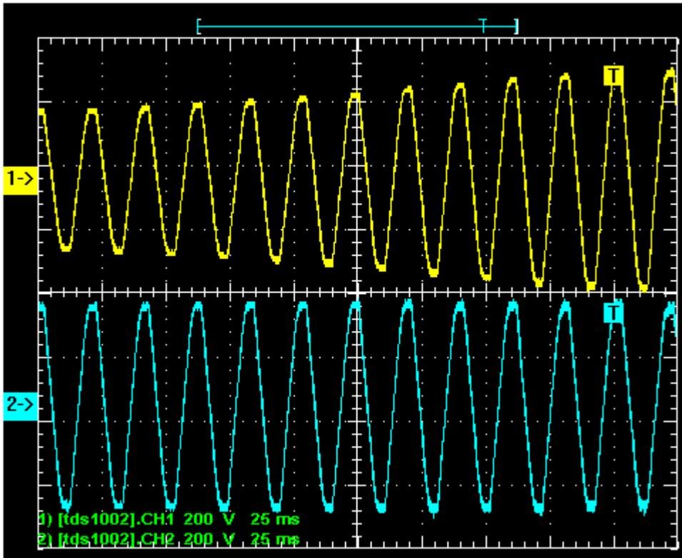
Input voltage (channel 1 – yellow) is dragged up from low voltage to high voltage within 0.2sec, but the output voltage (channel 2 - blue) remains steady.
